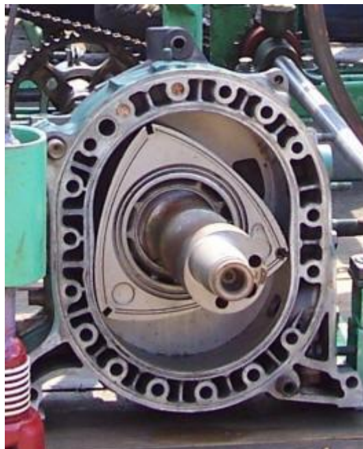
Figure 37 A Wankel rotary engine (Photo by J Lyon, Wikimedia Commons)
