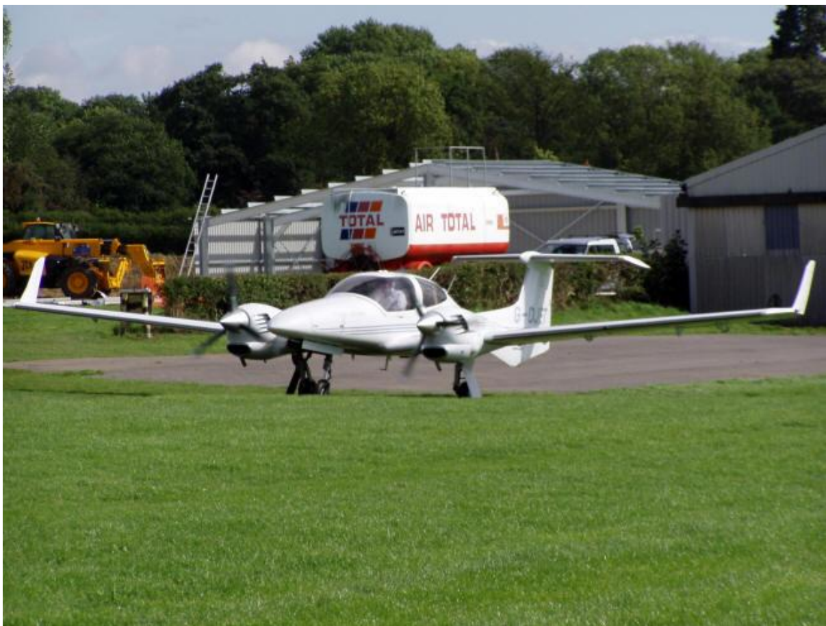
Figure 32 A piston-engine aircraft that runs on diesel fuel or Jet-A1
